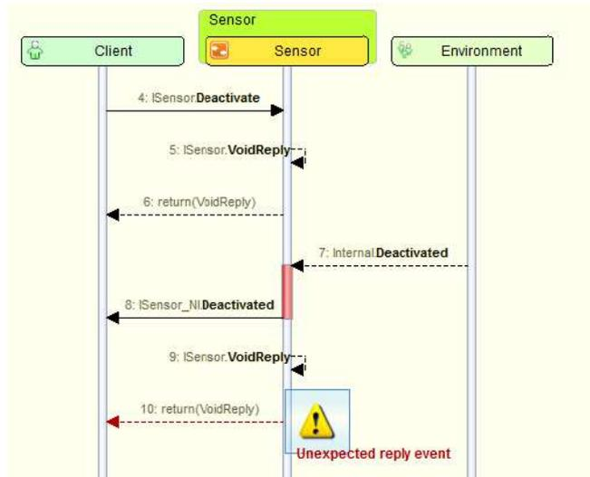
Failure trace in the "Sequence Diagram" tab showing an unexpected reply event
