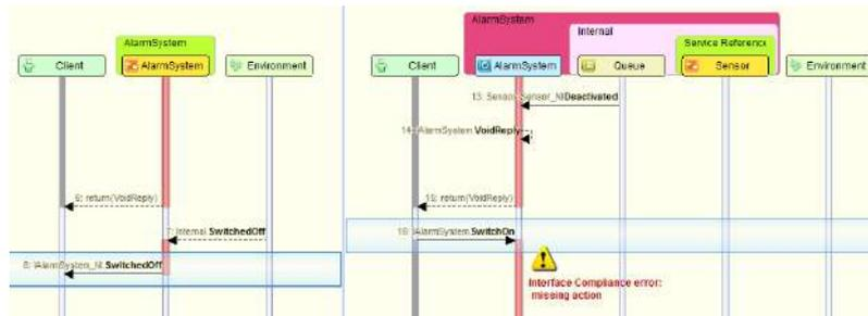
"Sequence Diagram" tab for interface compliance error
