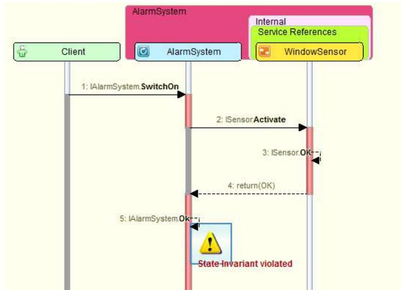
Failure trace in the "Sequence Diagram" tab showing a trace with a state invariant violation
