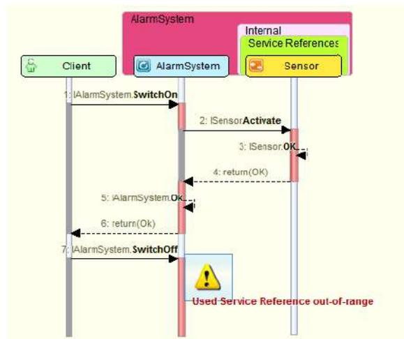
Failure trace in the "Sequence Diagram" tab showing a trace leading to range violation
