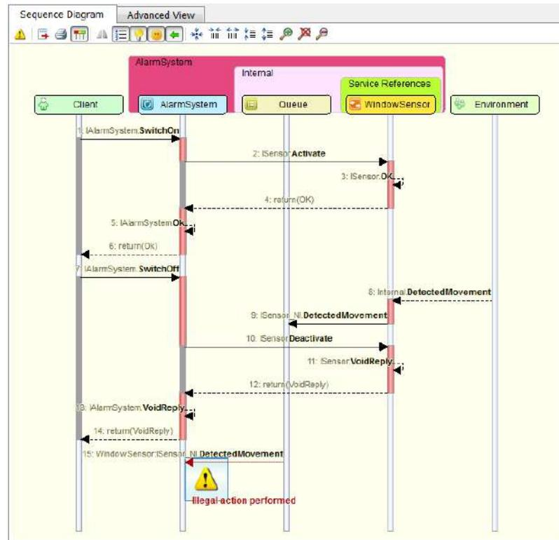
The "Sequence Diagram" tab of the "Visual Verification" window showing a failure trace
