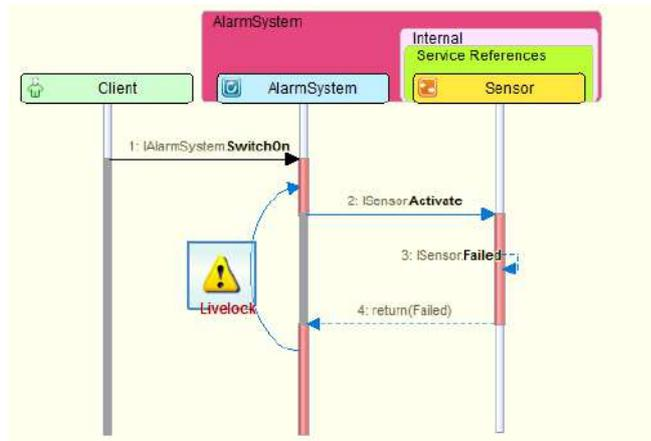
The "Visual Verification" window showing the infinite loop
