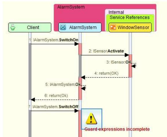
Failure trace in the "Sequence Diagram" tab showing a trace leading to an incomplete guard expression
