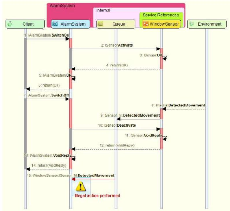
Failure trace in the "Sequence Diagram" tab showing a trace with an illegal action
