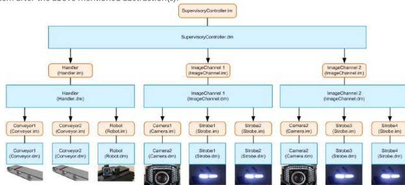
Component diagram for industrial visual inspection system - abstraction - first phase
