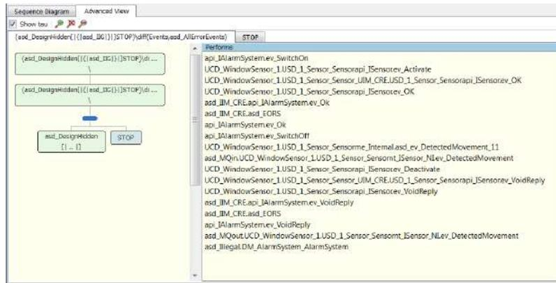
The "Advanced View" tab of the "Visual Verification" window showing a failure trace
